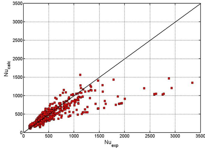
Figure 2: Experimental nusselt number versus calculated nusselt number using genetic algorithm minimization for plain tube data.
