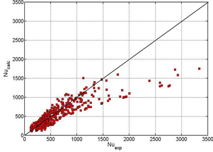
Figure 1: Experimental nusselt number versus Calculated nusselt number functional relation type 1
